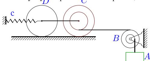
$$\begin{aligned}m_A &= 5 \text{ кг}, m_B = 3 \text{ кг}, m_C = 3 \text{ кг}, \\m_D &= 4 \text{ кг}, R_B = 9 \text{ см}, r_c = 8 \text{ см}, \\R_c &= 14 \text{ см}, i_c = 12 \text{ см}, r_B = 8 \text{ см}, \\i_B &= 8 \text{ см}, r_D = 14 \text{ см}, \delta_{fr} = 5 \text{ мм}, \\&c = 1 \text{ Н/м}.\end{aligned}$$
