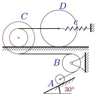
$$\begin{aligned} m_A &= 27 \text{ кг}, m_B = 138 \text{ кг}, m_C = 40 \text{ кг}, \\ m_D &= 90 \text{ кг}, R_B = 9 \text{ см}, r_c = 8 \text{ см}, \\ R_c &= 14 \text{ см}, i_c = 12 \text{ см}, r_D = 16 \text{ см}, \\ r_A &= 6 \text{ см}, \delta_{fr}=4 \text{ мм}, c = 1 \text{ Н/м}. \end{aligned}$$
