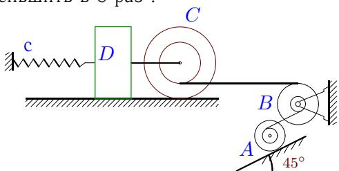
$$m_A = 35 \text{ кг}, m_B = 3 \text{ кг}, m_C = 6 \text{ кг}, \\ m_D = 12 \text{ кг}, R_B = 25 \text{ см}, r_c = 24 \text{ см}, \\ R_c = 42 \text{ см}, i_c = 28 \text{ см}, r_B = 24 \text{ см}, \\ i_B = 24 \text{ см}, r_A = 21 \text{ см}, R_A = 23 \text{ см}, \\ i_A = 22 \text{ см}, f = 0.05, \delta_{fr} = 9 \text{ мм}, c = 7 \text{ Н/м}.$$
