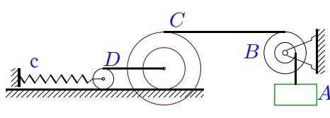
$$\begin{aligned} m_A &= 3 \text{ кг}, m_B = 3 \text{ кг}, m_C = 6 \text{ кг}, \\ m_D &= 8 \text{ кг}, R_B = 17 \text{ см}, r_c = 16 \text{ см}, \\ R_c &= 28 \text{ см}, i_c = 20 \text{ см}, r_B = 16 \text{ см}, \\ i_B &= 16 \text{ см}, r_D = 8 \text{ см}, \delta_{fr}=7 \text{ мм}, \\ c &= 2 \text{ Н/м}. \end{aligned}$$
