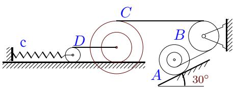
$$m_A = 2 \text{ кг}, m_B = 118 \text{ кг}, m_C = 80 \text{ кг}, \\ m_D = 30 \text{ кг}, R_B = 17 \text{ см}, r_c = 16 \text{ см}, \\ R_c = 28 \text{ см}, i_c = 20 \text{ см}, r_D = 8 \text{ см}, \\ r_A = 16 \text{ см}, R_A = 21 \text{ см}, i_A = 17 \text{ см}, \\ \delta_{fr} = 7 \text{ мм}, c = 87 \text{ Н/м}.$$
