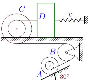
$$m_A = 2 \text{ кг}, m_B = 288 \text{ кг}, m_C = 80 \text{ кг}, \\ m_D = 90 \text{ кг}, R_B = 25 \text{ см}, r_c = 24 \text{ см}, \\ R_c = 42 \text{ см}, i_c = 28 \text{ см}, r_A = 22 \text{ см}, \\ R_A = 24 \text{ см}, i_A = 23 \text{ см}, f = 0.01, \\ \delta_{fr} = 8 \text{ мм}, c = 8 \text{ Н/м}.$$
