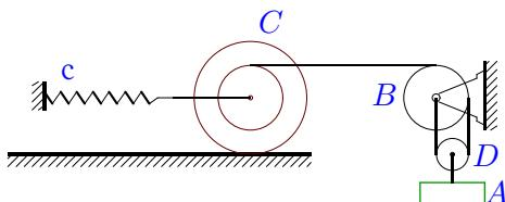
$$m_A = 11 \text{ кг}, m_B = 3 \text{ кг}, m_C = 9 \text{ кг}, \\ m_D = 12 \text{ кг}, R_B = 25 \text{ см}, r_c = 24 \text{ см}, \\ R_c = 42 \text{ см}, i_c = 28 \text{ см}, \delta_{fr} = 9 \text{ мм}, \\ c = 3 \text{ Н/м}.$$
