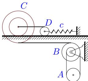
$$\begin{aligned}m_A &= 14 \text{ кг}, m_B = 12 \text{ кг}, m_C = 5 \text{ кг}, \\m_D &= 8 \text{ кг}, R_B = 17 \text{ см}, r_c = 16 \text{ см}, \\R_c &= 28 \text{ см}, i_c = 20 \text{ см}, r_B = 9 \text{ см}, \\i_B &= 16 \text{ см}, r_D = 8 \text{ см}, r_A = 13 \text{ см}, \\\delta_{fr} &= 7 \text{ мм}, c = 0.2 \text{ Н/м}.\end{aligned}$$
