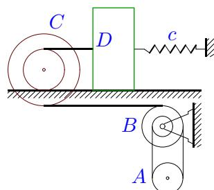
$$\begin{aligned} m_A &= 17 \text{ кг}, m_B = 3 \text{ кг}, m_C = 6 \text{ кг}, \\ m_D &= 12 \text{ кг}, R_B = 25 \text{ см}, r_c = 24 \text{ см}, \\ R_c &= 42 \text{ см}, i_c = 28 \text{ см}, r_B = 17 \text{ см}, \\ i_B &= 24 \text{ см}, r_A = 21 \text{ см}, f = 0.05, \delta_{fr} = 8 \text{ мм}, \\ c &= 0.3 \text{ Н/м}. \end{aligned}$$
