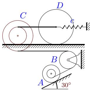
$$m_A = 9 \text{ кг}, m_B = 256 \text{ кг}, m_C = 40 \text{ кг}, \\ m_D = 90 \text{ кг}, R_B = 9 \text{ см}, r_c = 8 \text{ см}, \\ R_c = 14 \text{ см}, i_c = 12 \text{ см}, r_D = 16 \text{ см}, \\ r_A = 6 \text{ см}, R_A = 9 \text{ см}, i_A = 7 \text{ см}, \delta_{fr} = 4 \text{ мм}, \\ M_{fr.B} = 2 \text{ Нм}.$$
