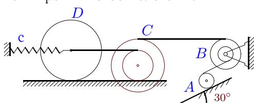
$$\begin{aligned}m_A &= 47 \text{ кг}, m_B = 12 \text{ кг}, m_C = 5 \text{ кг}, \\m_D &= 4 \text{ кг}, R_B = 9 \text{ см}, r_c = 8 \text{ см}, \\R_c &= 14 \text{ см}, i_c = 12 \text{ см}, r_B = 8 \text{ см}, \\i_B &= 8 \text{ см}, r_D = 16 \text{ см}, r_A = 8 \text{ см}, \\&\delta_{fr} = 4 \text{ мм}, c = 1 \text{ Н/м}.\end{aligned}$$
