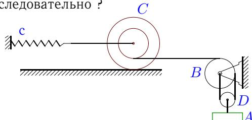
$$\begin{aligned} m_A &= 10 \text{ кг}, m_B = 6 \text{ кг}, m_C = 9 \text{ кг}, \\ m_D &= 4 \text{ кг}, R_B = 9 \text{ см}, r_c = 8 \text{ см}, \\ R_c &= 14 \text{ см}, i_c = 12 \text{ см}, r_D = R_B/2, \\ \delta_{fr} &= 5 \text{ мм}, M_{fr.B} = 4 \text{ Нм}. \end{aligned}$$
