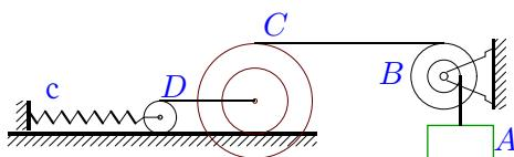
$$m_A = 3 \text{ кг}, m_B = 3 \text{ кг}, m_C = 5 \text{ кг}, \\ m_D = 8 \text{ кг}, R_B = 17 \text{ см}, r_c = 16 \text{ см}, \\ R_c = 28 \text{ см}, i_c = 20 \text{ см}, r_B = 16 \text{ см}, \\ i_B = 16 \text{ см}, r_D = 8 \text{ см}, \delta_{fr} = 7 \text{ мм}, \\ c = 2 \text{ Н/м}.$$
