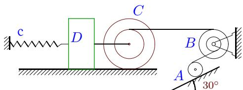
$$m_A = 10 \text{ кг}, m_B = 6 \text{ кг}, m_C = 3 \text{ кг}, \\ m_D = 12 \text{ кг}, R_B = 25 \text{ см}, r_c = 24 \text{ см}, \\ R_c = 42 \text{ см}, i_c = 28 \text{ см}, r_B = 24 \text{ см}, \\ i_B = 24 \text{ см}, r_A = 23 \text{ см}, f = 0.02, \delta_{fr} = 9 \text{ мм}, \\ M_{fr.B} = 4 \text{ Нм}.$$
