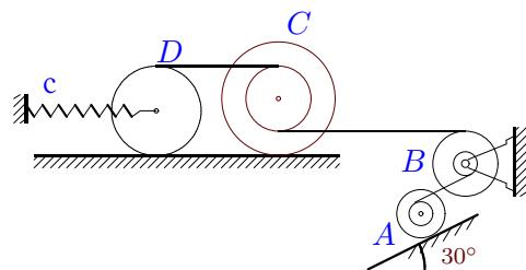
$$\begin{aligned} m_A &= 25 \text{ кг}, m_B = 3 \text{ кг}, m_C = 2 \text{ кг}, \\ m_D &= 8 \text{ кг}, R_B = 17 \text{ см}, r_c = 16 \text{ см}, \\ R_c &= 28 \text{ см}, i_c = 20 \text{ см}, r_B = 16 \text{ см}, \\ i_B &= 16 \text{ см}, r_D = 22 \text{ см}, r_A = 13 \text{ см}, \\ R_A &= 15 \text{ см}, i_A = 14 \text{ см}, \delta_{fr} = 6 \text{ мм}, \\ c &= 6 \text{ Н/м}. \end{aligned}$$
