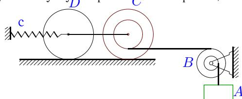
$$\begin{aligned} m_A &= 10 \text{ кг}, m_B = 9 \text{ кг}, m_C = 2 \text{ кг}, \\ m_D &= 4 \text{ кг}, R_B = 9 \text{ см}, r_c = 8 \text{ см}, \\ R_c &= 14 \text{ см}, i_c = 12 \text{ см}, r_B = 8 \text{ см}, \\ i_B &= 8 \text{ см}, r_D = 14 \text{ см}, \delta_{fr}=5 \text{ мм}, \\ M_{fr.B} &= 6 \text{ Нм}. \end{aligned}$$
