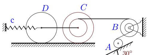
$$m_A = 26 \text{ кг}, m_B = 6 \text{ кг}, m_C = 5 \text{ кг}, \\ m_D = 4 \text{ кг}, R_B = 9 \text{ см}, r_c = 8 \text{ см}, \\ R_c = 14 \text{ см}, i_c = 12 \text{ см}, r_B = 8 \text{ см}, \\ i_B = 8 \text{ см}, r_D = 14 \text{ см}, r_A = 7 \text{ см}, \\ \delta_{fr} = 5 \text{ мм}, M_{fr.B} = 4 \text{ Нм}.$$
