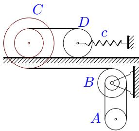
$$m_A = 12 \text{ кг}, m_B = 9 \text{ кг}, m_C = 6 \text{ кг}, \\ m_D = 8 \text{ кг}, R_B = 17 \text{ см}, r_c = 16 \text{ см}, \\ R_c = 28 \text{ см}, i_c = 20 \text{ см}, r_B = 9 \text{ см}, \\ i_B = 16 \text{ см}, r_D = 16 \text{ см}, r_A = 13 \text{ см}, \\ \delta_{fr} = 6 \text{ мм}, M_{fr.B} = 3 \text{ Нм}.$$
