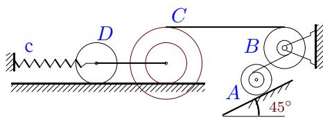
$$\begin{aligned} m_A &= 12 \text{ кг}, m_B = 6 \text{ кг}, m_C = 7 \text{ кг}, \\ m_D &= 4 \text{ кг}, R_B = 9 \text{ см}, r_c = 8 \text{ см}, \\ R_c &= 14 \text{ см}, i_c = 12 \text{ см}, r_B = 8 \text{ см}, \\ i_B &= 8 \text{ см}, r_D = 8 \text{ см}, r_A = 8 \text{ см}, \\ R_A &= 11 \text{ см}, i_A = 9 \text{ см}, \delta_{fr} = 5 \text{ мм}, \\ M_{fr.B} &= 3 \text{ Нм}. \end{aligned}$$
