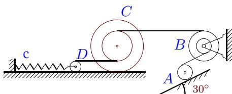
$$\begin{aligned}m_A &= 7 \text{ кг}, m_B = 3 \text{ кг}, m_C = 2 \text{ кг}, \\m_D &= 8 \text{ кг}, R_B = 17 \text{ см}, r_c = 16 \text{ см}, \\R_c &= 28 \text{ см}, i_c = 20 \text{ см}, r_B = 16 \text{ см}, \\i_B &= 16 \text{ см}, r_D = 6 \text{ см}, r_A = 15 \text{ см}, \\\delta_{fr} &= 6 \text{ мм}, c = 2 \text{ Н/м}.\end{aligned}$$
