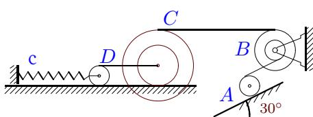
$$\begin{aligned}m_A &= 24 \text{ кг}, m_B = 12 \text{ кг}, m_C = 5 \text{ кг}, \\m_D &= 8 \text{ кг}, R_B = 17 \text{ см}, r_c = 16 \text{ см}, \\R_c &= 28 \text{ см}, i_c = 20 \text{ см}, r_B = 16 \text{ см}, \\i_B &= 16 \text{ см}, r_D = 8 \text{ см}, r_A = 16 \text{ см}, \\&\delta_{fr} = 7 \text{ мм}, c = 2 \text{ Н/м}.\end{aligned}$$
