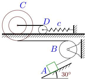
$$\begin{aligned}m_A &= 29 \text{ кг}, m_B = 36 \text{ кг}, m_C = 80 \text{ кг}, \\m_D &= 90 \text{ кг}, R_B = 17 \text{ см}, r_c = 16 \text{ см}, \\R_c &= 28 \text{ см}, i_c = 20 \text{ см}, r_D = 8 \text{ см}, f = 0.03, \\&\delta_{fr} = 7 \text{ мм}, M_{fr,B} = 5 \text{ Нм}.\end{aligned}$$
