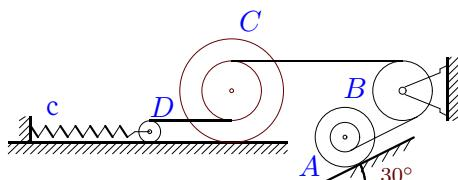
$$\begin{aligned} m_A &= 2 \text{ кг}, m_B = 196 \text{ кг}, m_C = 60 \text{ кг}, \\ m_D &= 60 \text{ кг}, R_B = 17 \text{ см}, r_c = 16 \text{ см}, \\ R_c &= 28 \text{ см}, i_c = 20 \text{ см}, r_D = 6 \text{ см}, \\ r_A &= 15 \text{ см}, R_A = 19 \text{ см}, i_A = 16 \text{ см}, \\ \delta_{fr} &= 6 \text{ мм}, M_{fr.B} = 1 \text{ Нм}. \end{aligned}$$
