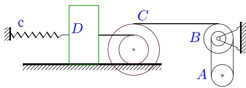
$$\begin{aligned} m_A &= 7 \text{ кг}, m_B = 6 \text{ кг}, m_C = 2 \text{ кг}, \\ m_D &= 12 \text{ кг}, R_B = 25 \text{ см}, r_c = 24 \text{ см}, \\ R_c &= 42 \text{ см}, i_c = 28 \text{ см}, r_B = 17 \text{ см}, \\ i_B &= 24 \text{ см}, r_A = 21 \text{ см}, f = 0.01, \delta_{fr} = 8 \text{ мм}, \\ M_{fr.B} &= 2 \text{ Нм}. \end{aligned}$$
