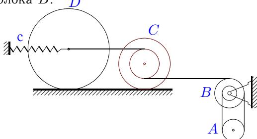
$$m_A = 13 \text{ кг}, m_B = 12 \text{ кг}, m_C = 8 \text{ кг}, \\ m_D = 4 \text{ кг}, R_B = 9 \text{ см}, r_c = 8 \text{ см}, \\ R_c = 14 \text{ см}, i_c = 12 \text{ см}, r_B = 1 \text{ см}, \\ i_B = 8 \text{ см}, r_D = 22 \text{ см}, r_A = 5 \text{ см}, \\ \delta_{fr} = 4 \text{ мм}, c = 0.1 \text{ Н/м}.$$
