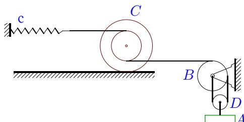
$$\begin{aligned} m_A &= 9 \text{ кг}, m_B = 12 \text{ кг}, m_C = 9 \text{ кг}, \\ m_D &= 8 \text{ кг}, R_B = 17 \text{ см}, r_c = 16 \text{ см}, \\ R_c &= 28 \text{ см}, i_c = 20 \text{ см}, r_D = R_B/2, \\ \delta_{fr} &= 6 \text{ мм}, c = 2 \text{ Н/м}. \end{aligned}$$
