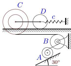
$$\begin{aligned} m_A &= 39 \text{ кг}, m_B = 12 \text{ кг}, m_C = 5 \text{ кг}, \\ m_D &= 4 \text{ кг}, R_B = 9 \text{ см}, r_c = 8 \text{ см}, \\ R_c &= 14 \text{ см}, i_c = 12 \text{ см}, r_B = 8 \text{ см}, \\ i_B &= 8 \text{ см}, r_D = 8 \text{ см}, r_A = 6 \text{ см}, \\ R_A &= 11 \text{ см}, i_A = 7 \text{ см}, \delta_{fr} = 5 \text{ мм}, \\ c &= 4 \text{ Н/м}. \end{aligned}$$
