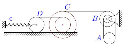
$$\begin{aligned} m_A &= 10 \text{ кг}, m_B = 9 \text{ кг}, m_C = 9 \text{ кг}, \\ m_D &= 8 \text{ кг}, R_B = 17 \text{ см}, r_c = 16 \text{ см}, \\ R_c &= 28 \text{ см}, i_c = 20 \text{ см}, r_B = 9 \text{ см}, \\ i_B &= 16 \text{ см}, r_D = 16 \text{ см}, r_A = 13 \text{ см}, \\ \delta_{fr} &= 6 \text{ мм}, M_{fr.B} = 3 \text{ Нм}. \end{aligned}$$
