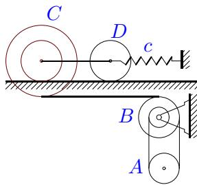
$$\begin{aligned} m_A &= 11 \text{ кг}, m_B = 9 \text{ кг}, m_C = 6 \text{ кг}, \\ m_D &= 4 \text{ кг}, R_B = 9 \text{ см}, r_c = 8 \text{ см}, \\ R_c &= 14 \text{ см}, i_c = 12 \text{ см}, r_B = 1 \text{ см}, \\ i_B &= 8 \text{ см}, r_D = 8 \text{ см}, r_A = 5 \text{ см}, \delta_{fr} = 5 \text{ мм}, \\ M_{fr.B} &= 3 \text{ Нм}. \end{aligned}$$
