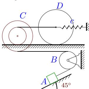
$$\begin{aligned}m_A &= 18 \text{ кг}, m_B = 21 \text{ кг}, m_C = 40 \text{ кг}, \\m_D &= 90 \text{ кг}, R_B = 9 \text{ см}, r_c = 8 \text{ см}, \\R_c &= 14 \text{ см}, i_c = 12 \text{ см}, r_D = 16 \text{ см}, \\f &= 0.06, \delta_{fr} = 4 \text{ мм}, c = 1 \text{ Н/м}.\end{aligned}$$
