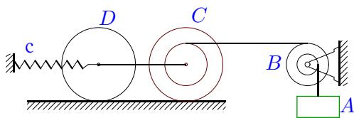
$$m_A = 12 \text{ кг}, m_B = 12 \text{ кг}, m_C = 7 \text{ кг}, \\ m_D = 4 \text{ кг}, R_B = 9 \text{ см}, r_c = 8 \text{ см}, \\ R_c = 14 \text{ см}, i_c = 12 \text{ см}, r_B = 8 \text{ см}, \\ i_B = 8 \text{ см}, r_D = 14 \text{ см}, \delta_{fr} = 5 \text{ мм}, \\ c = 1 \text{ Н/м}.$$
